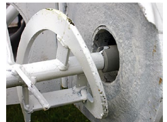
7 Connect the transport and the mixing screw to each other. (Keep coupling clean - never lubricate)
