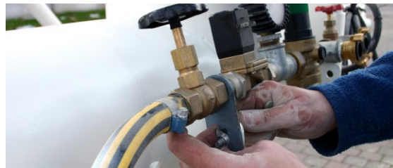
9 Store the water fitting for protection against frost and theft. (Caution: if this not observed, the repair will be charged).
