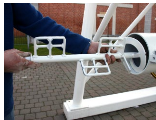
5 Pull out mixing screw completely and clean it.
