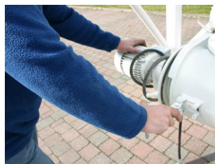
1 Open the closing piece with the motor.
