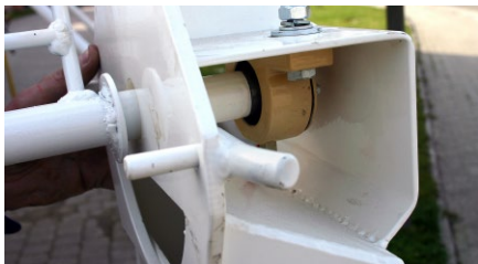
8 Replace the end piece of the mixing tube. (Play between bearing and mixing screw should not exceed 2 mm )
