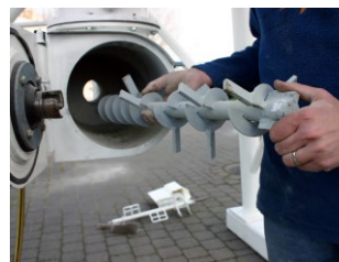
2 Clean the conveyor screw and the dry chamber without using water.
