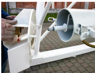
4 Remove the end piece from the mixer tube.
