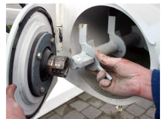
3 Replace the transport screw in the cleaned motor coupling and close the dry chamber.
