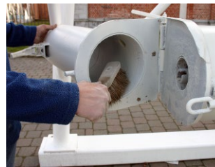
6 Open and clean the mixing tube (do not wet the dry chamber). Replace the mixing tube and the mixing screw.
